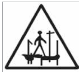
Danger Scaffolding Incomplete
